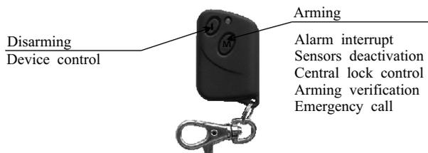
Fig. 3. Two-button remote control.
